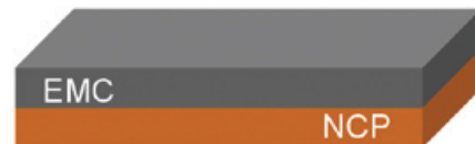
Figure 2. EMC/NCP bi-material joint
